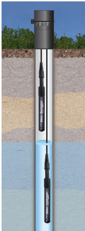
for use in air, making this instrument extremely accurate. The barometric data is then used, along with a software Wizard, to compensate the Levellogger data, and provide true water level readings. To increase the accuracy of barometric compensation data, it is recommended the Barologger and Levelloggers be programmed with the same recording times.
