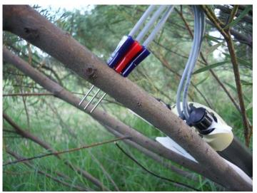
The HRM needles have two radial measurement points for the charaterisation of radial sap flow gradients making measurements more accurate. Through microprocessor control, the inner measurement point can be activated or deactivated dependent on the specific wood anatomy of the species being measured. This provides a great flexibility in stem diameter range from >10 mm diameter woody stems or roots to the world's largest Redwood trees.
