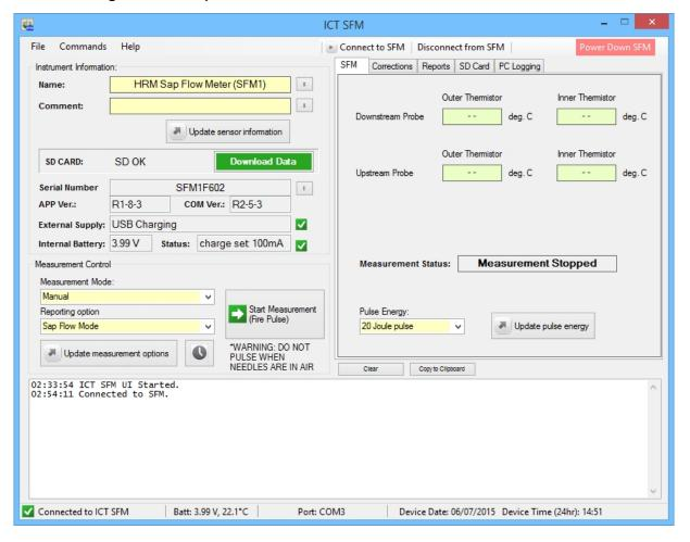
All aspects of the instrument's operation and calculations are controlled by the microprocessor, which automatically converts the analogue microvolt signals to a calibrated output. Programming variables such as heat pulse interval, energy input, probe spacings, and measurement frequency are all stored in non-volatile memory.
