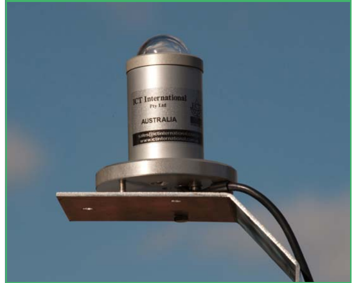
SK-08 sensor measuring solar radiation across India
