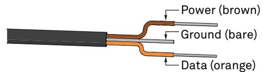
NOTE: Sensors manufactured as MPS-6 use white wire for power and red wire for data output.
