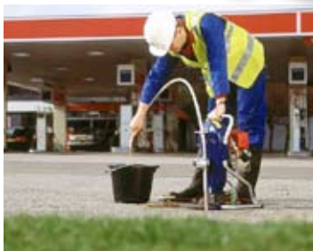
PowerPack PP1 over flush-fitting borehole. PowerPack PP1 back-pack frame.
