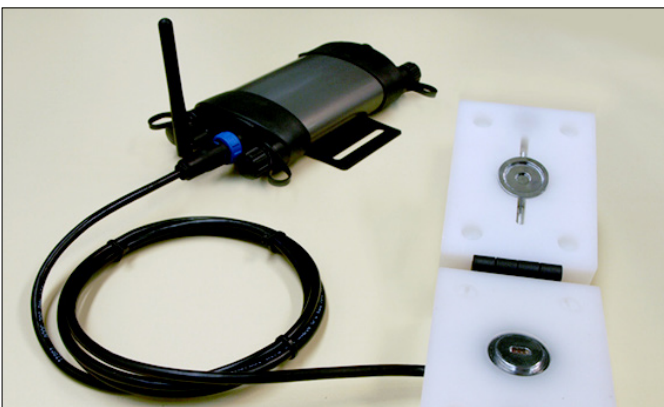
Figure 4.1., 4.2., 4.3. The PSY1 Stem Psychrometer chamber embedded in the Osmotic Potential Insulator
