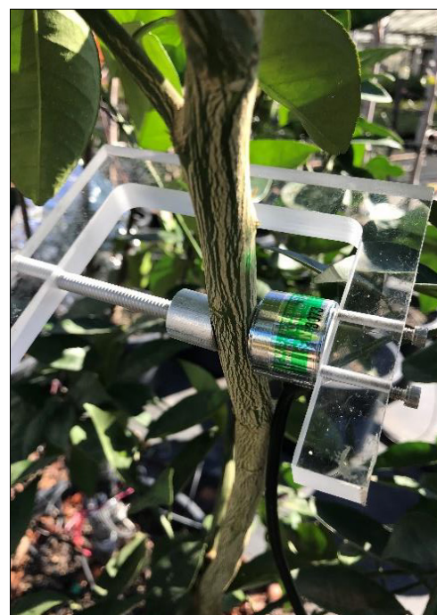
Figure 18. Installed PSY1-Stem sensor on citrus stem
