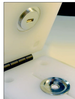
Figures 23.1., 23.2. The psychrometer chamber mounted inside the Osmotic Potential Insulator (OPI) with loaded filter paper disc soaked in an extracted sap solution to measure osmotic potential
