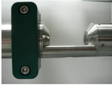
Mechanical sensor-holding system (front view)
