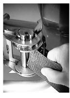
2. Take the strap around the circumference of the borehole lining or headworks and pass it through the ratchet slot. Pull tightly to remove slack (see picture).
