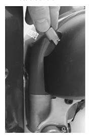
To adjust the throttle setting, move lever (indicated in the picture) anti-clockwise to slow the engine or clockwise to speed it up.
