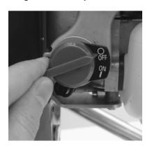
The Stop/Start switch is located on the side of the engine, near the fuel tank filler cap. (See picture on page 9)
