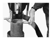
Check all components are secure. Check for loose fixings. Inspect clamping strap for wear (see picture).
