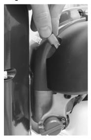
The throttle control and the Stop/Start switch are located on the side of the engine, near the fuel tank filler cap. (See picture)
