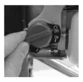
Start/Stop Switch: In an emergency, to switch off engine, turn knob to off position (O).
