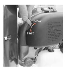
1. Position the throttle control lever fully to SLOW. This stops the actuator operating.
