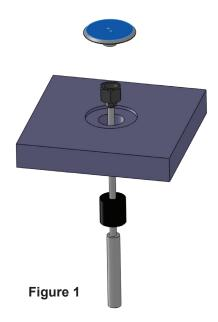
Then use a 1" masonry bit to bore through the remainder of the slab until sub-slab is reached. A 3" deep hole in the sub-slab is required so that the entire length of the screen can be exposed to the sub-slab.
