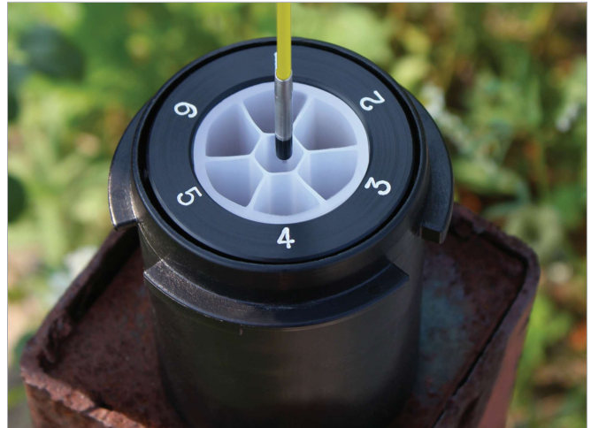
Measure water levels within the narrow channels of a Solinst CMT® System.
