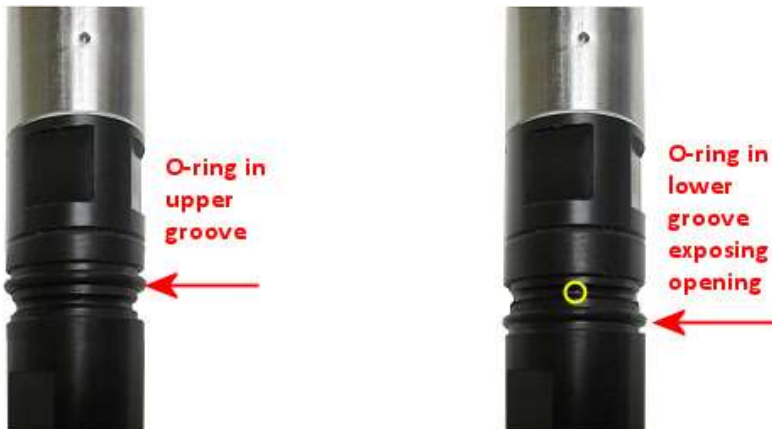
Be sure to move the o-ring to the lower groove before deploying, thus exposing the liquid junction port.
