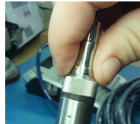
Properly completed—black ring uncompressed
