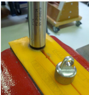
Cableless Sensor—gripping on knurled area
