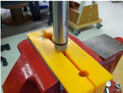
Cabled Sensor—gripping on swage
