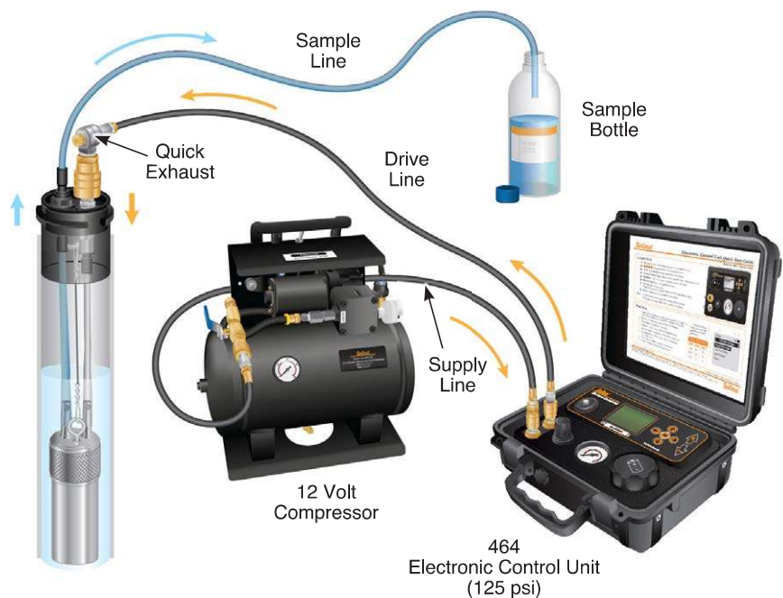
Figure 3-1 Pumping Set Up
