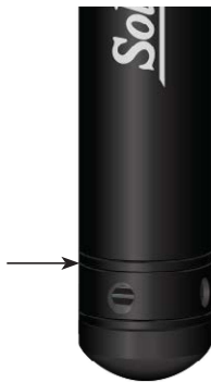
Figure 8-6 Logger Measurement Line
