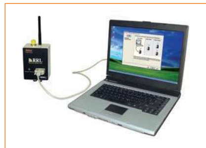
RRL Station connected to PC using RS232 cable
