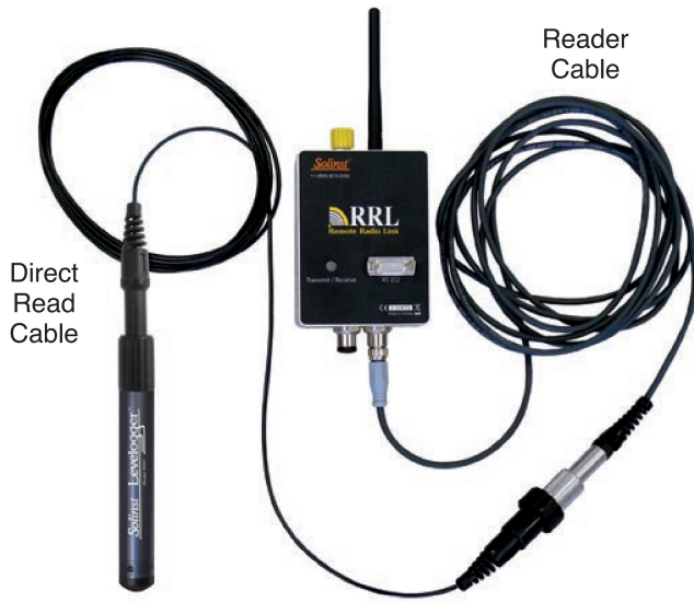
Levellogger Connection to the RRL Station
