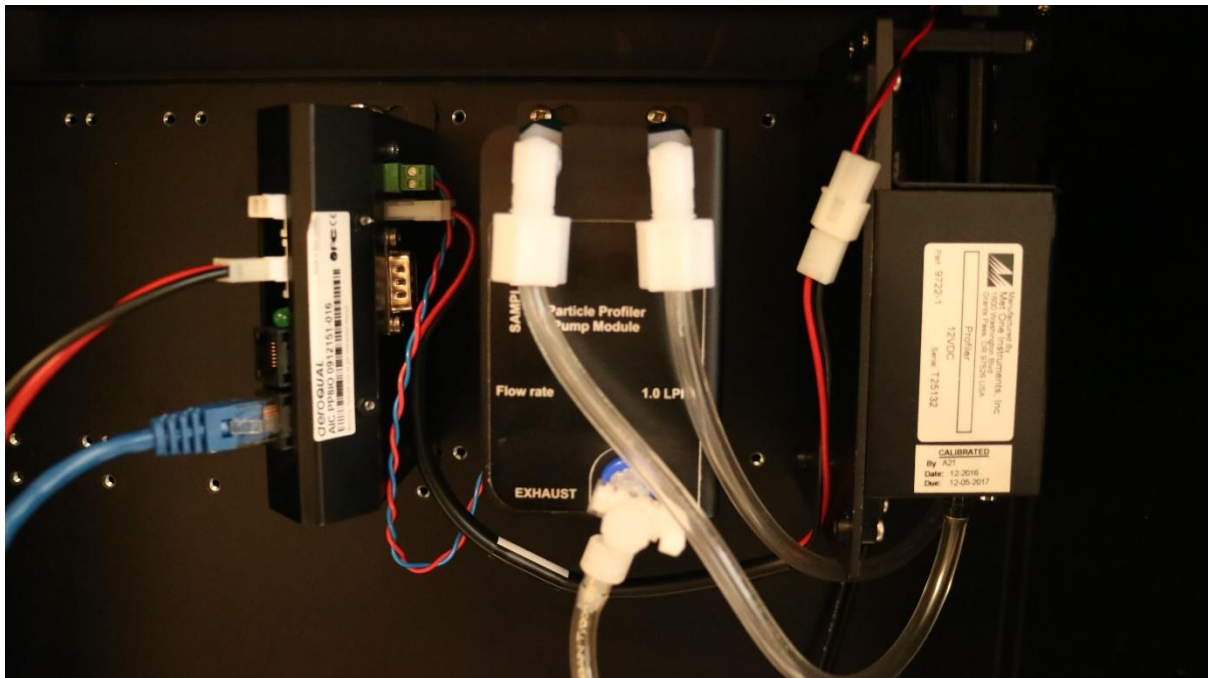
Figure 0-17 An update to the pump module with the filters installed inside the pump module
