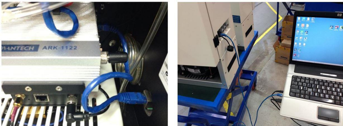
Figure 0-4 To establish a direct connection, a laptop must be connected to the ePC using an Ethernet cable
