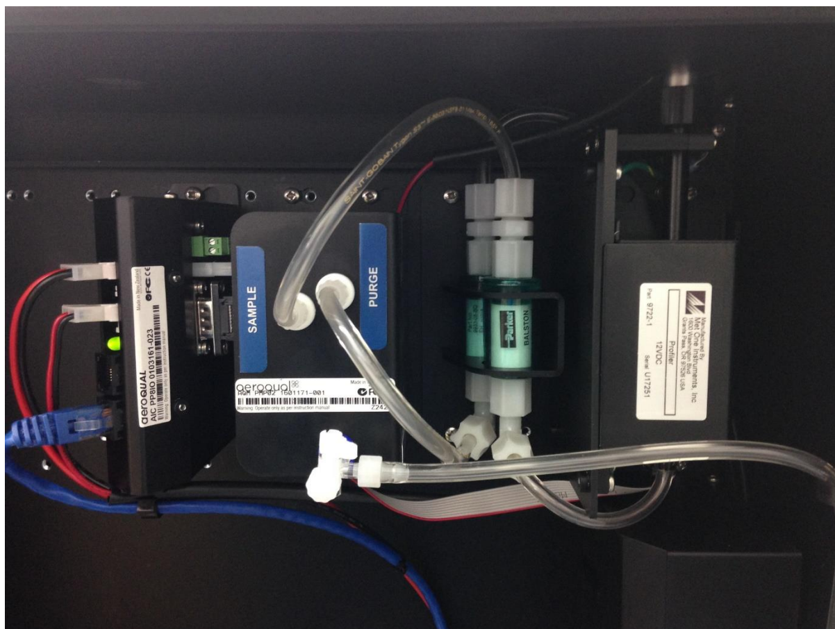
Figure 0-16 The Particle Profiler uses three modules: a) the optical module on the far right, b) the pump module in the middle, c) the electronics module on the left. The image above is the arrangement prior to July / August 2018.
