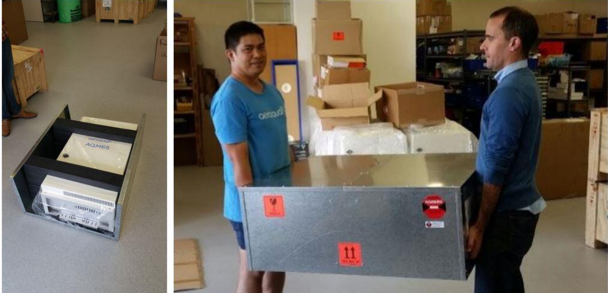
Figure 0-1 The total weight of the AQM 65 in its shipping container is about 65 kg (150 lbs).
