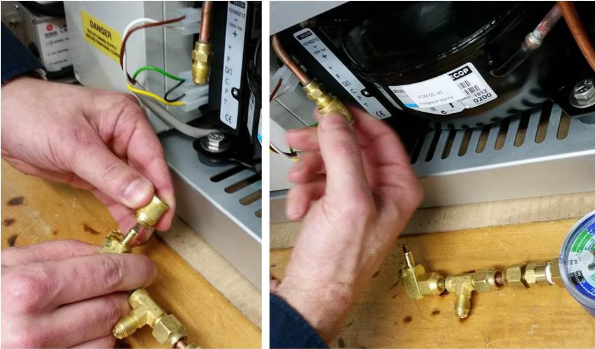
Figure 0-37 Attach the charging cap from the pressure gauge and screw it on to the gas inlet on the compressor
