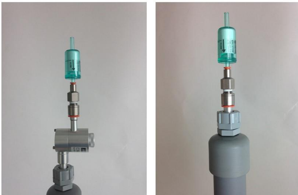
Figure 0-22 The zero filter is fitted above the cyclone for a Particle Monitor (left) and directly on the inlet for a Particle Profiler (right)
