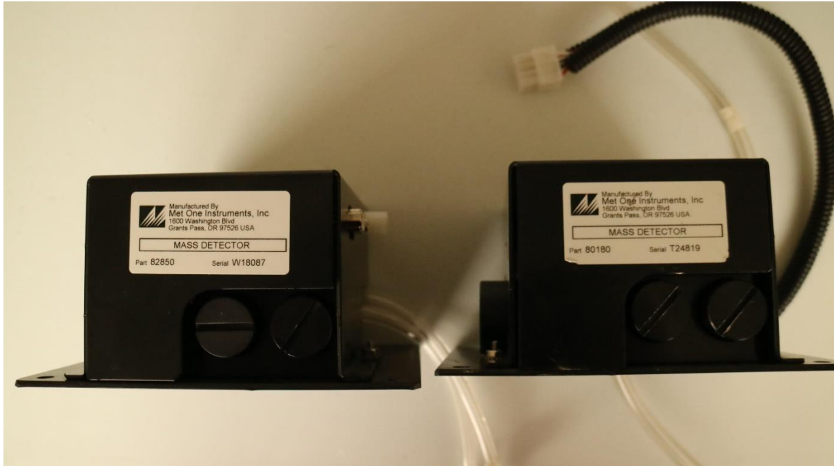
Figure 0-13 Left: 82850 optical module, Right 80180 optical module, the size and form factor are identical
