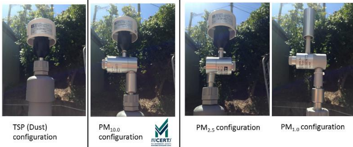
Figure 0-12 Size selection in the Particle Monitor is determined by the sharp cut cyclone on the inlet
