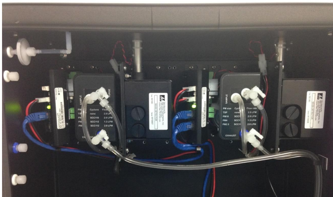
Figure 0-11 Two Particle Monitors can be installed in an AQM 65, each Particle Monitor will have three modules each
