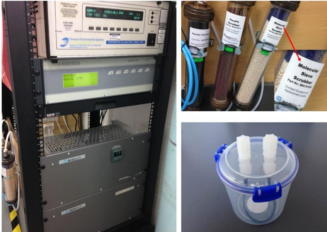
Figure 0-3 Left: Ecotech and Teledyne calibration system. Top Right: Drying agent molecular Sieves. Bottom right: Aeroqual R41 humidifier.
