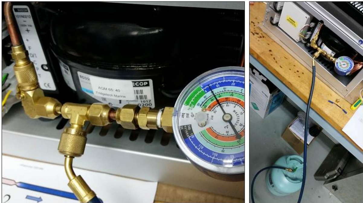
Figure 0-39 Hose attached to the pressure gauge and to the cylinder of R134a
