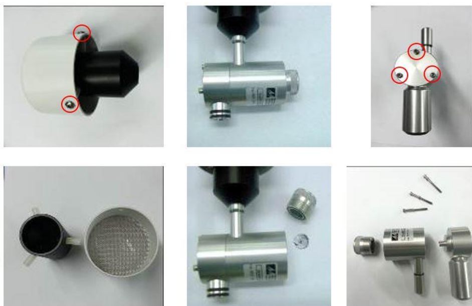
Figure 0-27 The TSP head and cyclone can be disassembled for cleaning
