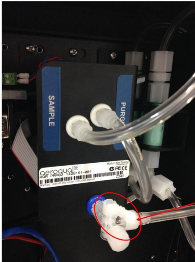
Figure 0-18 The flow rate of the Particle Profiler is set by adjusting the flow adjustment valve
