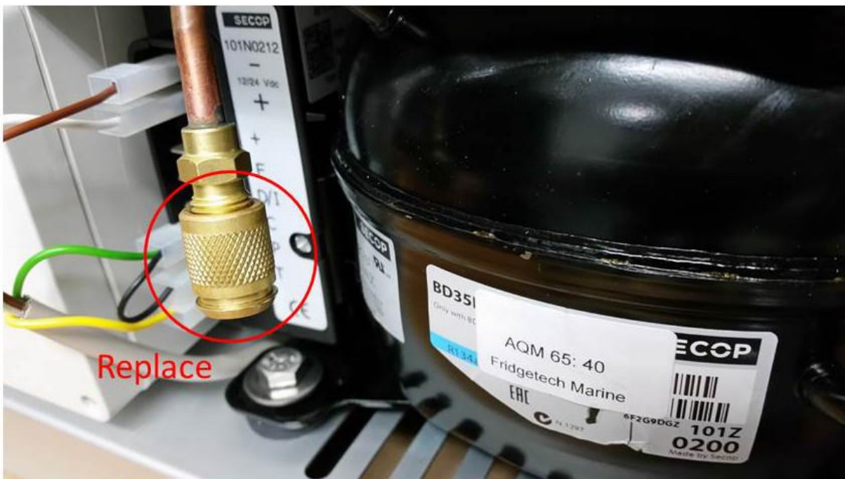
Figure 0-42 Replace the protection cap once you have finished the process
