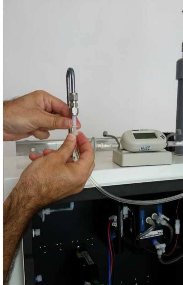
Figure 0-6 To measure the flow rate, remove the inlet filter and attach the inlet flow adaptor.
