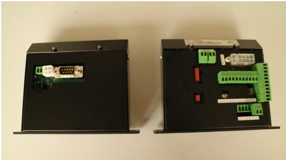
Figure 0-14 Left IO module for the 82850 optical module, note that the fiber span switch is no longer used, Right IO module for the 80180 optical module
