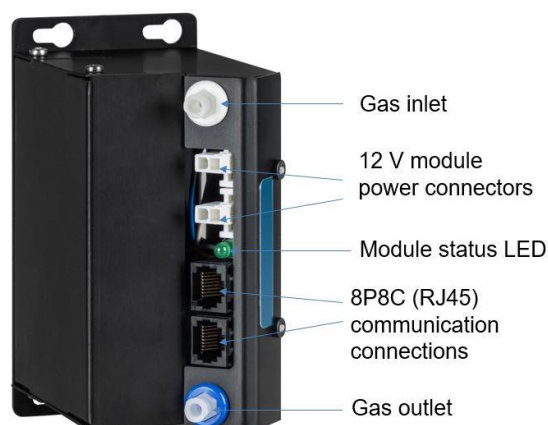
Figure 0-4 Gas sensor module with key components labelled
