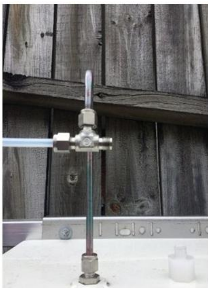
Figure 0-6 The AQM CALKIT connects the output of the AirCal 1000 to the input of the AQM 65 via a tee.
