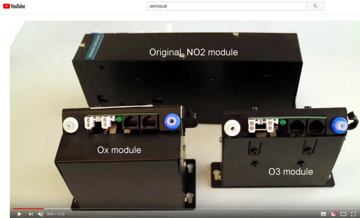
Figure 0-5 Replacing NO 2 module with O x /O 3 system for measuring NO 2 www.youtube.com/watch?v=4GS7ey4S-68
