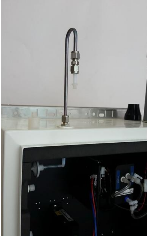
Figure 0-6 To measure the flow rate, remove the inlet filter and attach the inlet flow adaptor.
