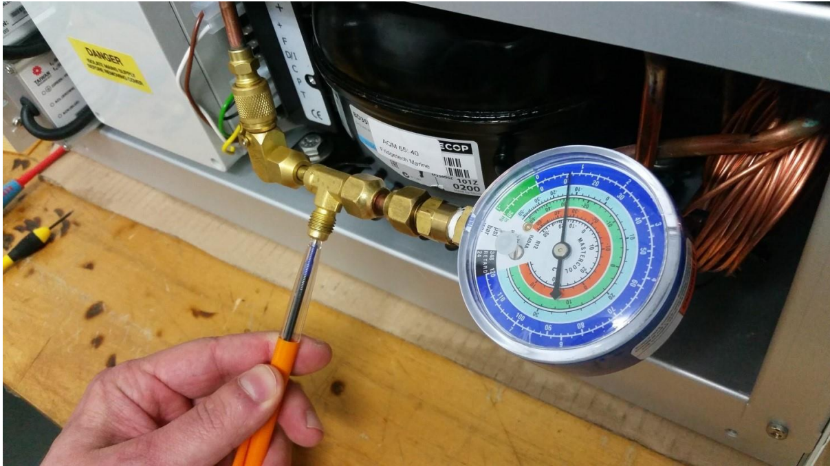
Figure 0-41 Gently release pressure from the gas line by pressing the release valve on the gauge
