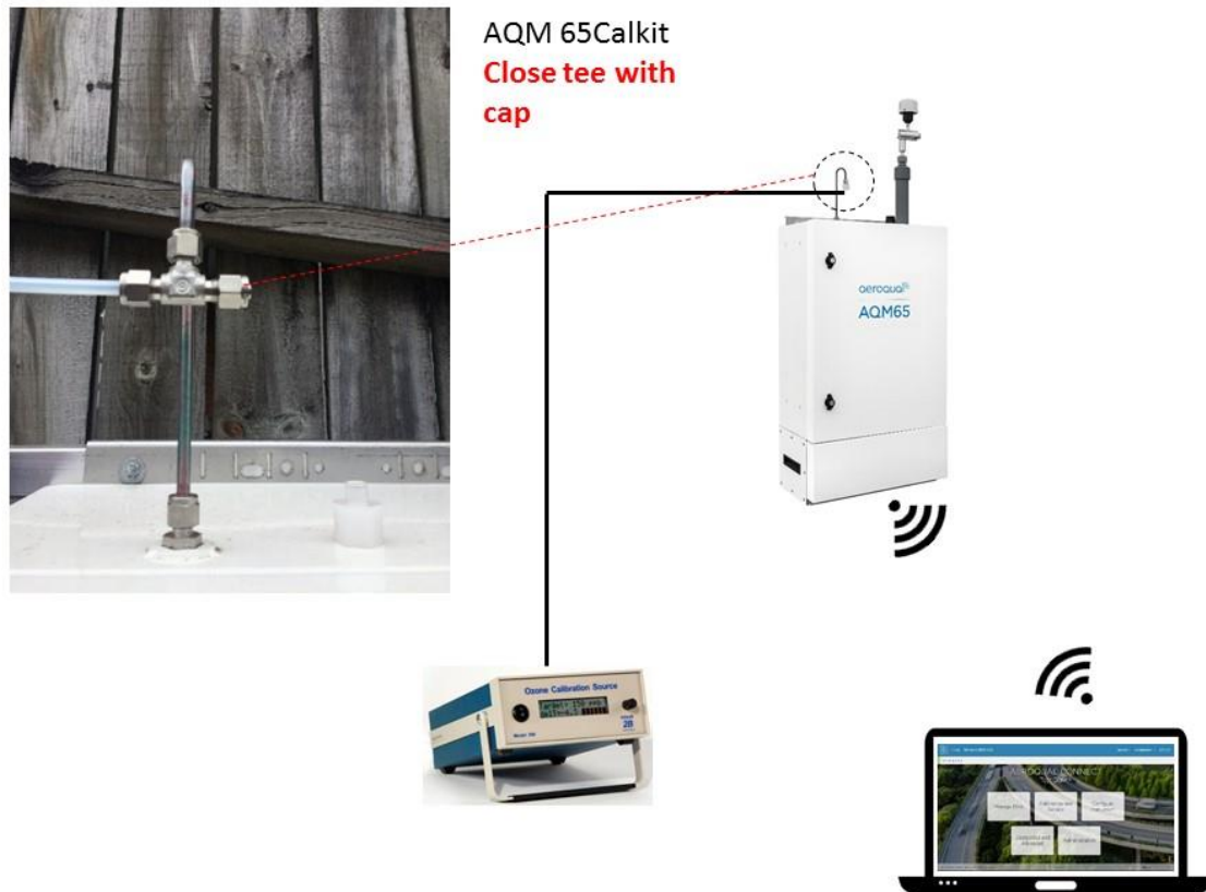
Figure 0-13 Setup to perform span calibration with Ozone calibrator
