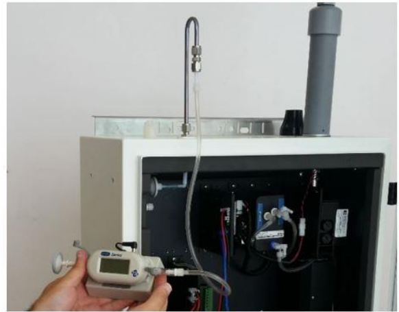
Figure 0-11 Connect inlet to AQM 65 and measure the flow rate to determine if connection is secure
