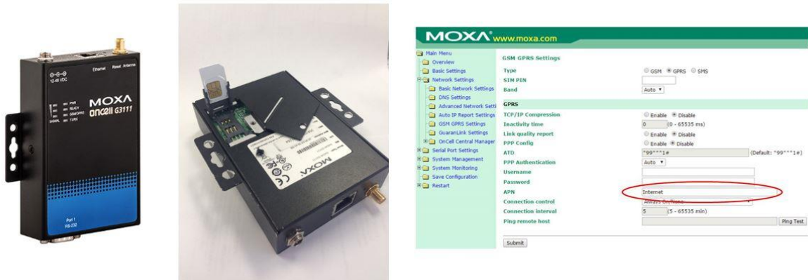
Figure 0-5 The MOXA modem uses a SIM card and it must be configured for use with the AQM 65
