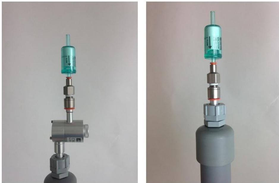
Figure 6-18 The zero filter is fitted above the cyclone for a Particle Monitor (left) and directly on the inlet for a Particle Profiler (right)
