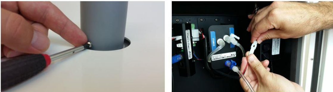
Figure 2-6 During field installation, secure the PM inlet using the retaining screws, then plug in the heater
