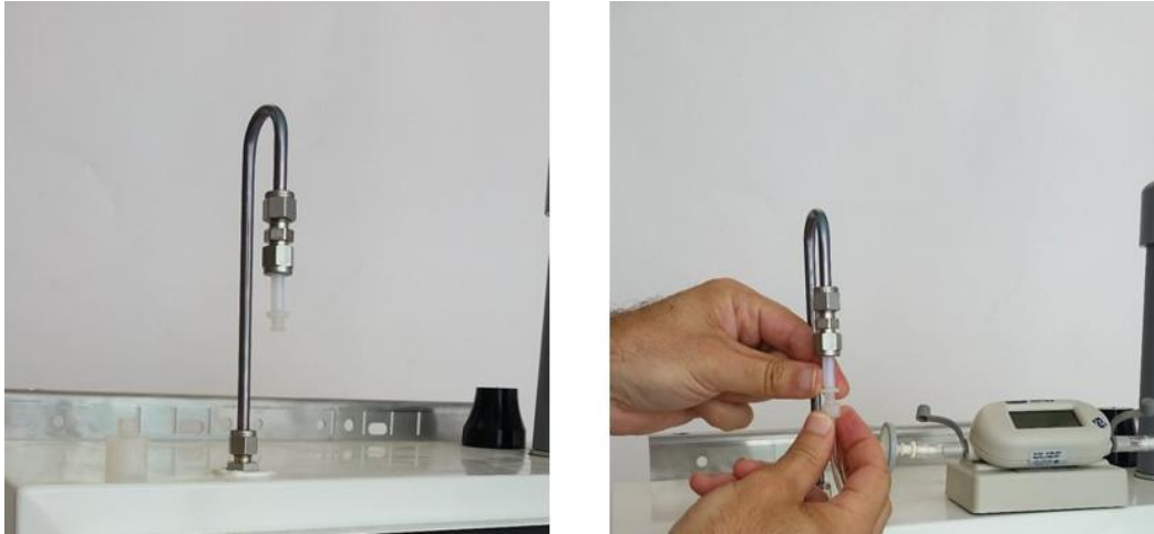
Figure 6-7 To measure the flow rate, remove the Kynar inlet filter and attach the inlet flow adaptor.
