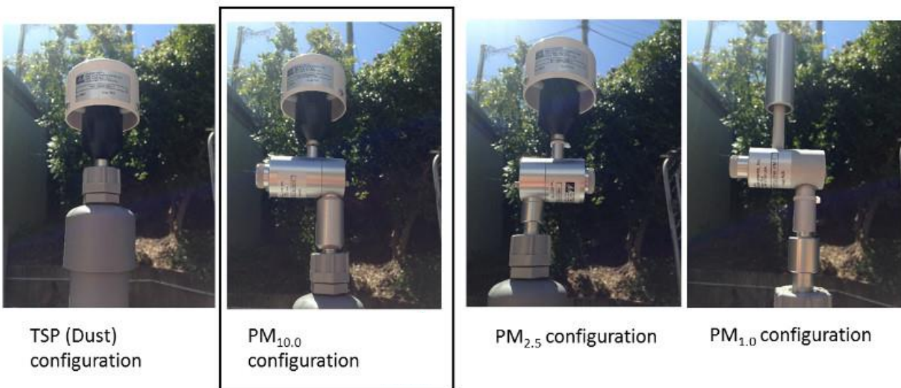
Figure 12-5 The size selection in the Particle Monitor is determined by the sharp cut cyclone on the inlet.
