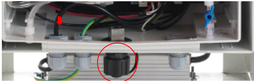
Figure 4-8 To establish a direct connection, a laptop must be connected to the ePC using an Ethernet cable
