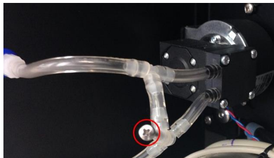
Figure 6-8 The flow adaptor valve is used to adjust the monitor inlet flow to the correct value.
