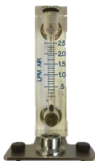
Figure 6-3 DS R8, 0.2 - 2.5 L/min rotameter for PM flow measurements.
