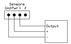
Three wire current loop sensors require power and ground connections to provide power to the sensor. The sensor output is wired to the appropriate input port.
