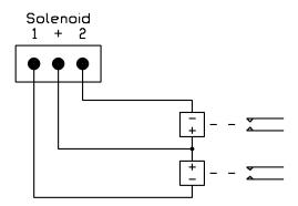
Alternatively, the digital outputs may be used as "NPN open-collector" drivers with pullup resistors provided by the attached device. The pullup resistor must not be taken to a voltage higher than the battery voltage of the CR unit.
