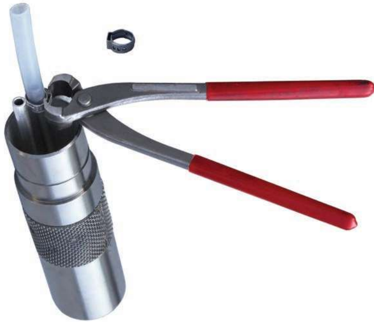
Figure 6-4 1/2"OD x 3/8"ID tubing attached to Port Stem Using Oetiker #14 Clamp
