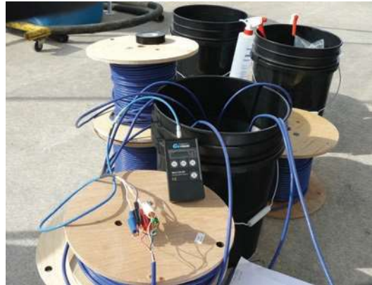
Figure 6-6 Presoaking the Vibrating Wire Transducers
