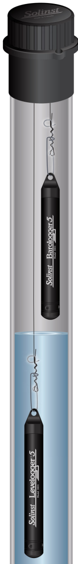
Figure 10-18 Levellogger and Barologger in Well
