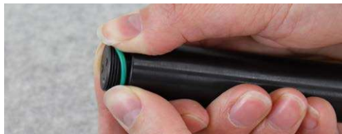
Figure 10-26 Replacing Levellogger O-rings
