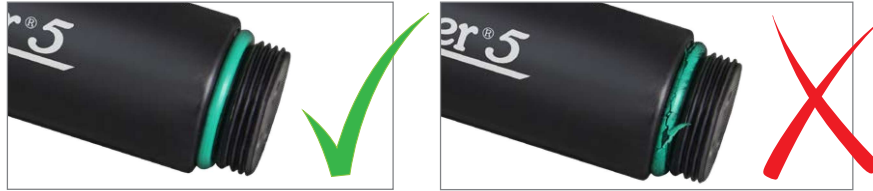
Figure 10-25 Levellogger O-ring Damage
