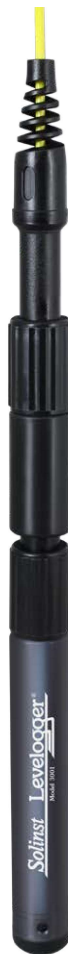
Figure 10-11 Levellogger Edge Connected to L5 Direct Read Cable Using an Edge–L5 DRC Adaptor
