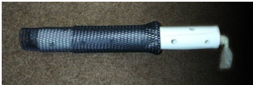
Figure 5-5. Dialysis sampler with rigid perforated support internal to the dialysis membrane. (1.25 inches in diameter by 14 inches long)
