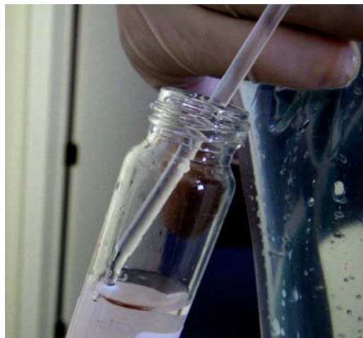
Figure 3-11. Discharging sample from HydraSleeve.
