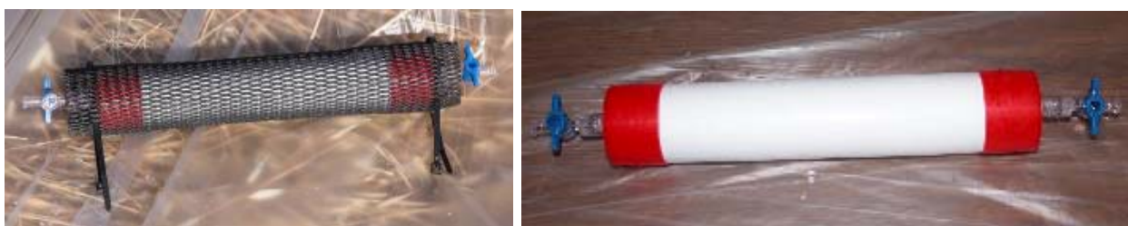
Figure 6-1. Original RPP design by Vroblesky with caps and valves at both ends.
