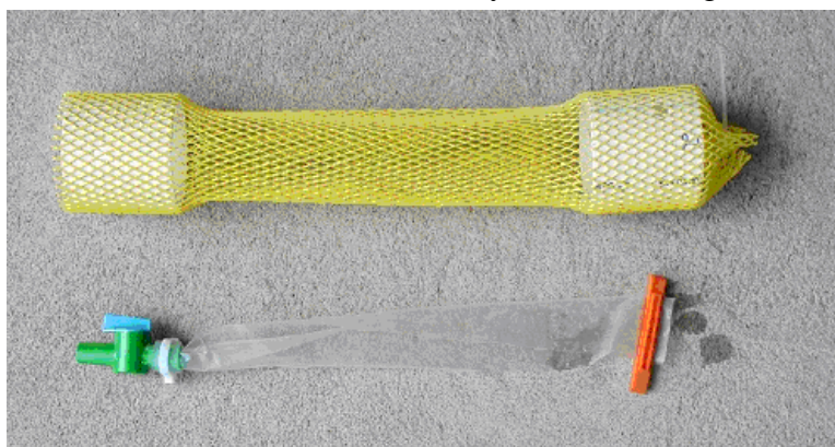
Figure 5-3. Partially assembled dialysis sampler before filling with deionized water with external supports installed in the protective mesh. (~2.5 inches in diameter by 24 inches long)
