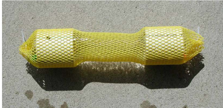
Figure 5-4. Fully assembled dialysis sampler with supports external to the dialysis membrane. (2.5 inches in diameter by 14 inches long)
