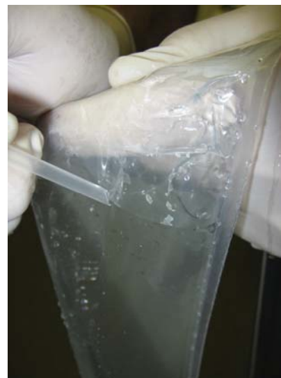
Figure 3-10. HydraSleeve flexible reed valve.
