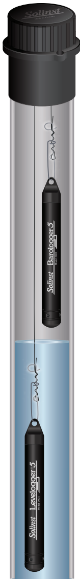
Figure 10-18 Levellogger and Barologger in Well
