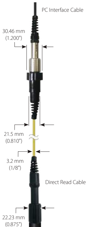
Figure 10-8 L5 Direct Read Cable Dimensions
