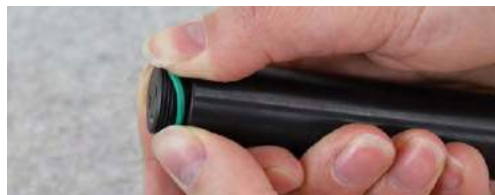
Figure 10-26 Replacing Levellogger O-rings
