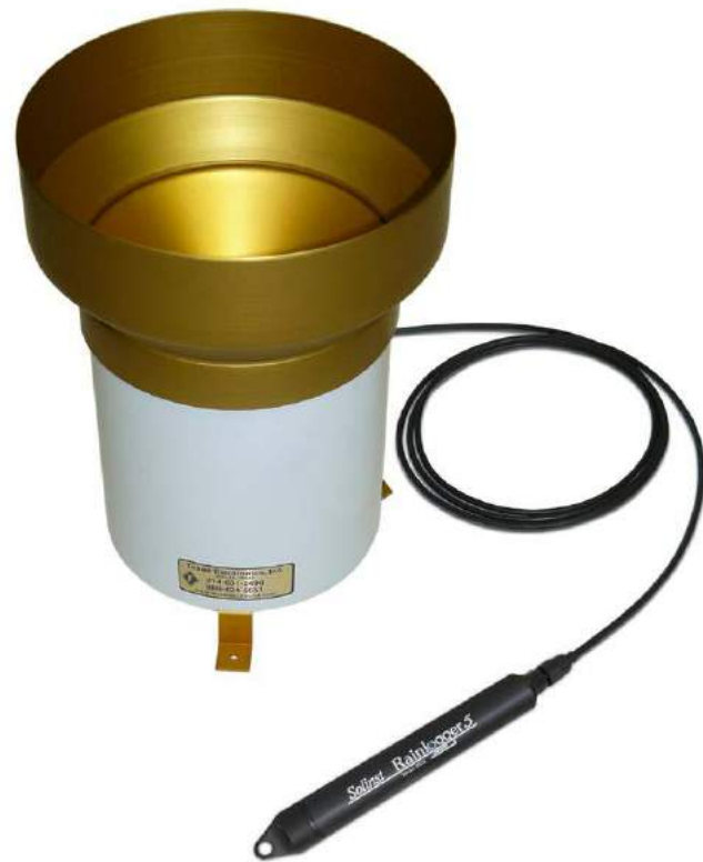
Figure 10-21 Rainlogger 5 Connected to Tipping-bucket
