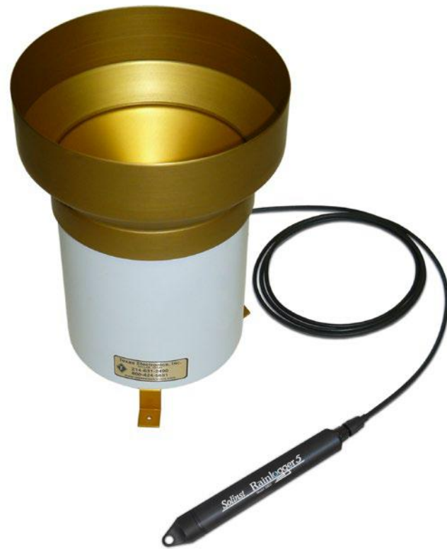
Figure 10-21 Rainlogger 5 Connected to Tipping-bucket
