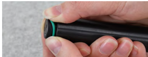
Figure 10-26 Replacing Levellogger O-rings
