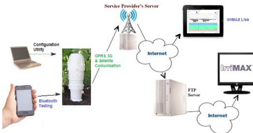
Figure 1 Block Diagram of the Sentek All-in-One in use
