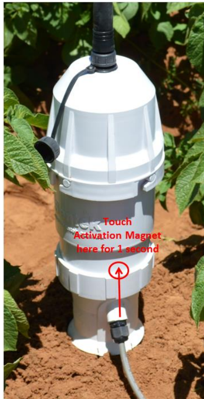
Figure 24 All-in-One Magnet switch position
