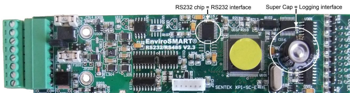
Figure 37 EnviroSCAN RS232 logging interface
