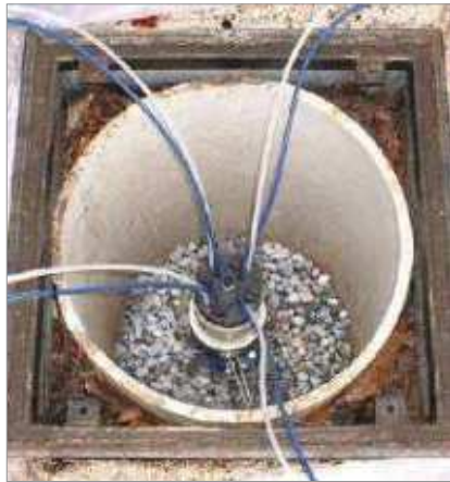
Using core logs to identify placement of Ports and Packers (left). Multi-Purge Manifold with transducers and dedicated pumps for four zone monitoring (right).
