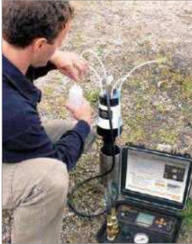
Collecting a sample from a dedicated DVP and taking pressure measurements with Model 404 Geokon Vibrating Wire Readout.
