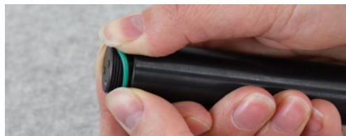
Figure 10-26 Replacing Levellogger O-rings
