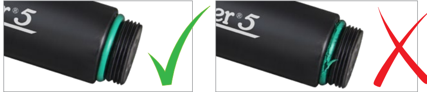
Figure 10-25 Levellogger O-ring Damage
