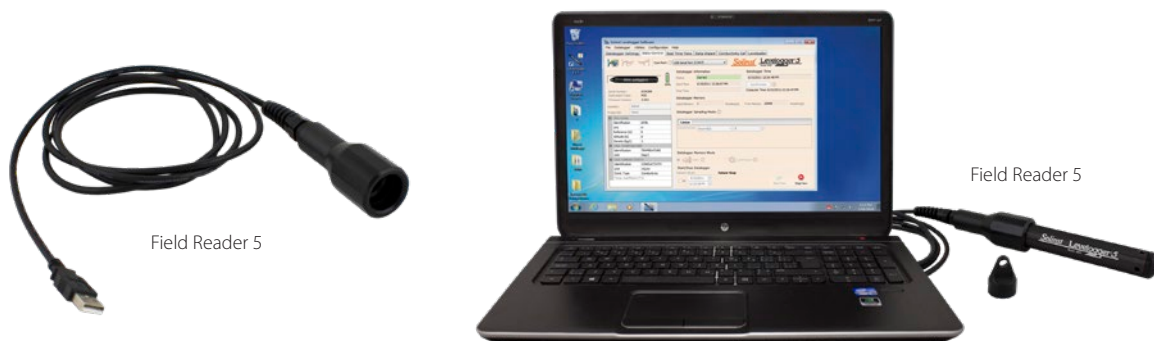
Figure 2-2 Levelogger 5 Connected to a PC Using a Field Reader 5
