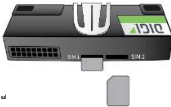
Figure 3-7 Inserting SIM Card
