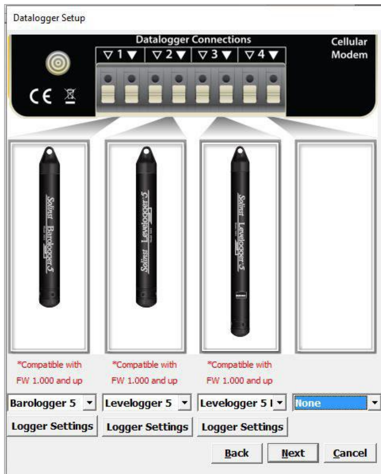
Figure 4-4 Datalogger Setup Window
