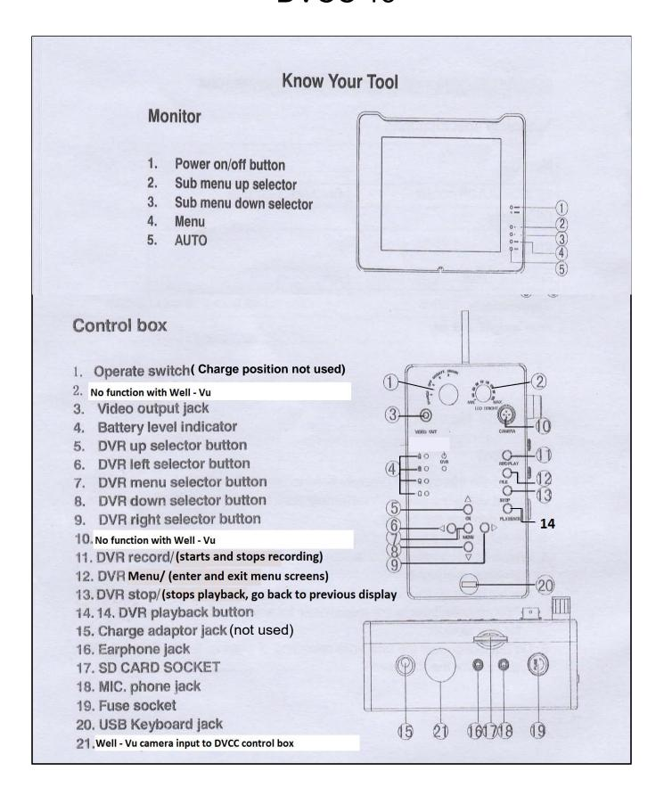
Note: When battery level indicator flashes, you have 90 seconds to save recorded data or images will be lost.
