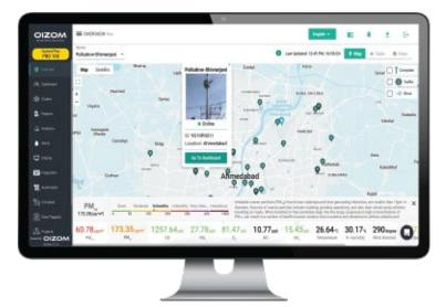
Envizom<sup>™</sup> is an Environmental monitoring software for real-time air quality data acquisition, visualization, and analytics. The Oizom<sup>®</sup> environmental data interpretation engine fetches the data from the Oizom<sup>®</sup> Environmental monitoring stations. On receiving the data, the engine runs necessary corrections and compensation algorithms. Envizom<sup>™</sup> uses secured HTTPS servers for data storage. Alternatively, this data can also be stored on-premise local servers.
