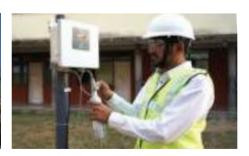
All air quality monitoring systems are calibrated at the ISO/IEC 17025:2017 certified calibration laboratory using standard NIST traceable calibration gas standards as per the international guidelines by USEPA.
