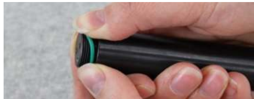
Figure 10-26 Replacing Levellogger O-rings
