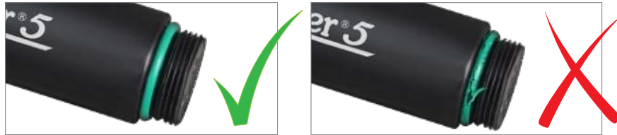
Figure 10-25 Levellogger O-ring Damage
