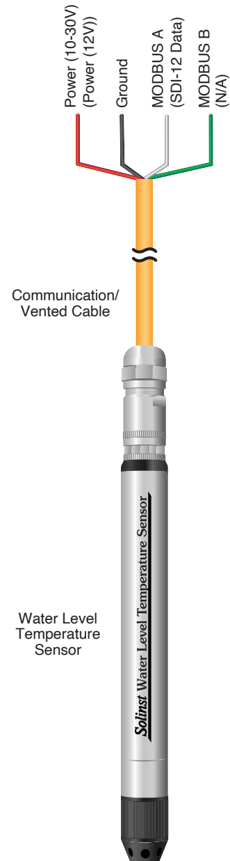
MODBUS Wiring Overview (SDI-12 in Brackets)
