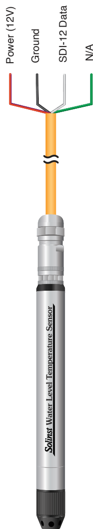
Figure 3-1 WLTS SDI-12 Wiring Overview
