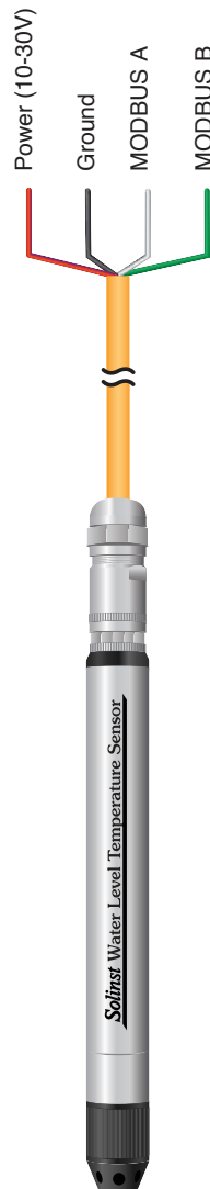
Figure 3-1 MODBUS Wiring Overview
