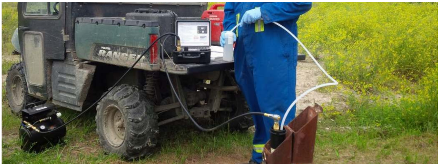
Groundwater Sampling with a Dedicated Bladder Pump using Portable, Rugged, Easy-to-use, Compressor and Controller
