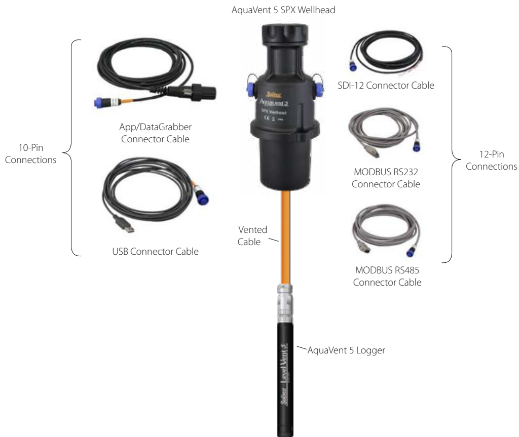
Figure 1-8 Complete AquaVent 5 System
