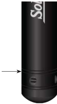
Figure 8-6 Logger Measurement Line
