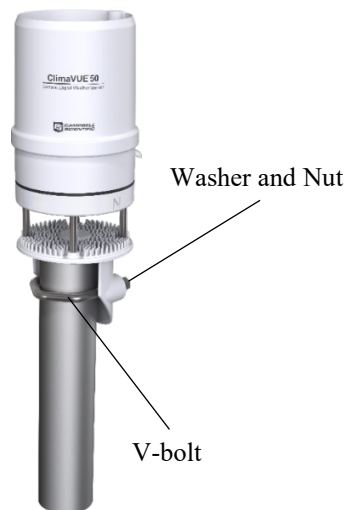
FIGURE 7-2. ClimaVUE 50 mounted to a pole with V-bolt and nuts
