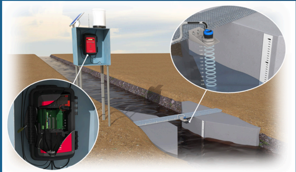
Flume and Weir applications
