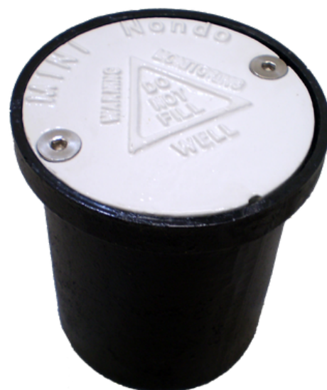
Mini Nondo Well Cover: Small cover ideal for soil vapour installations. Only 150mm OD, 124mm ID, 150mm cast iron skirt, Flush mount, bolt down lid, oring sealed.
