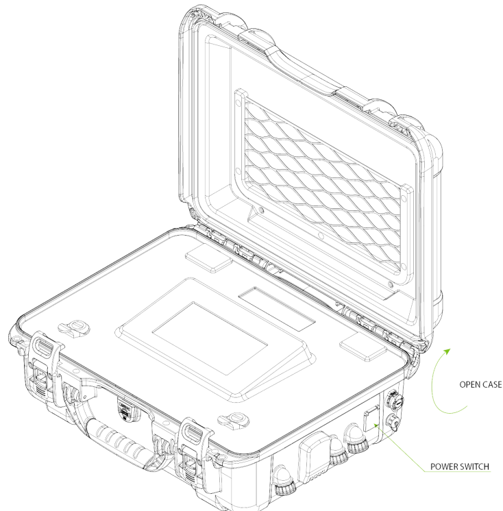
Figure 4.8 Open Case & Power Switch
