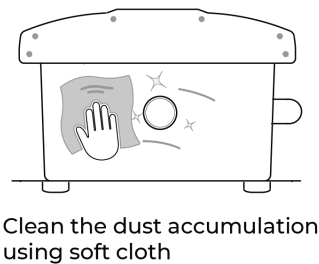
Figure 9.3 : Cleaning of UVL Sensor Dome
