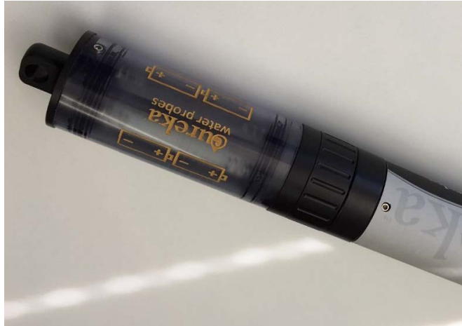
Figure 5-7 External Battery Pack Connected
