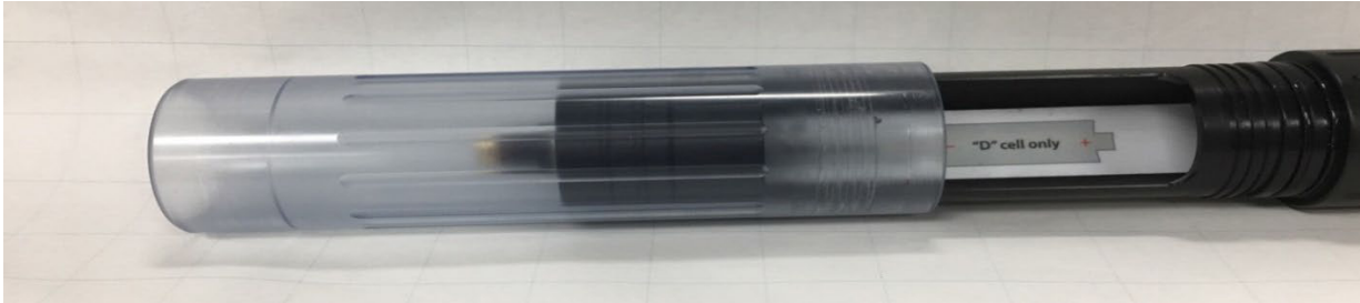
Figure 5-2 Manta 20/25/Trimeter Internal Battery Housing
