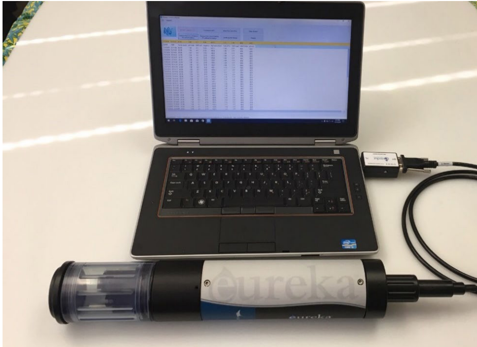
Figure 1-6 Manta Connected to a PC
