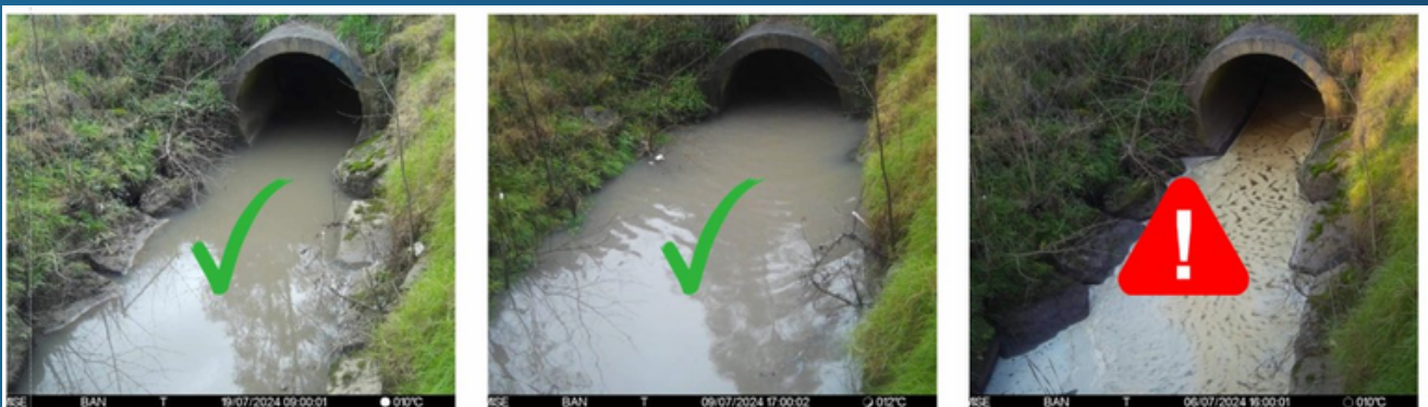
Automated detection: clean flow (left, centre) versus a flagged pollution event (right).
