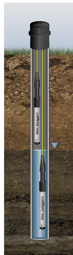
Barologger and Levellogger installed in Well Using Direct Read Cables
