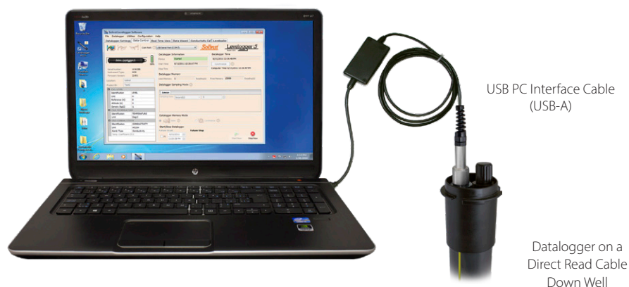
Figure 2-7 Datalogger and Direct Read Cable Connected to PC Using a PC Interface Cable
