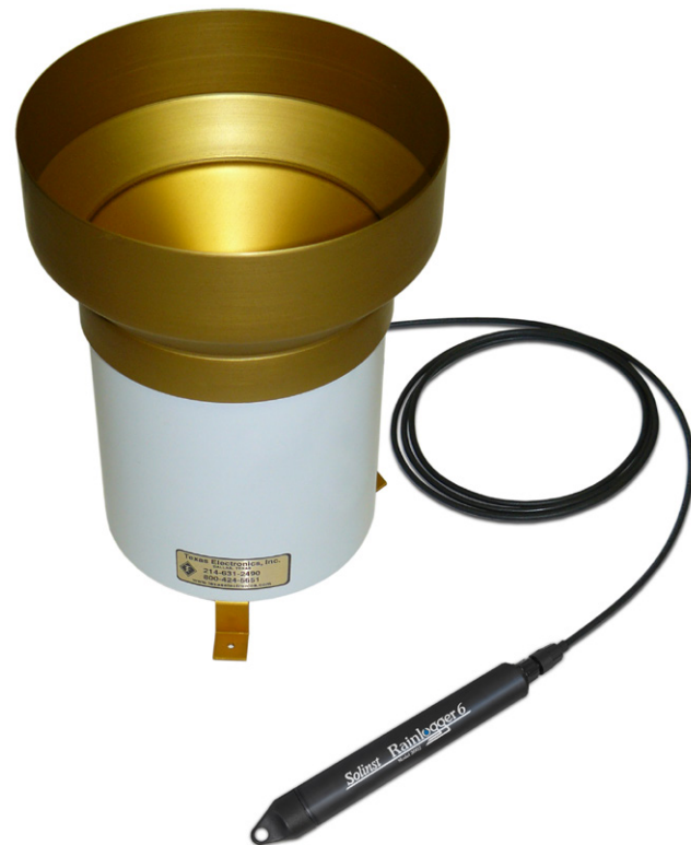
Figure 10-21 Rainlogger 6 Connected to Tipping-bucket
