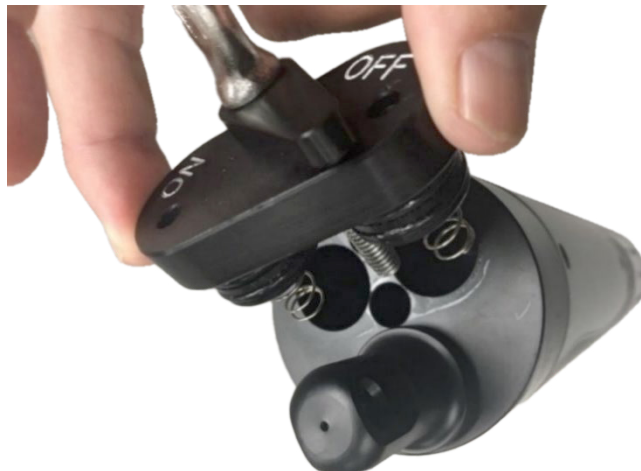
Figure 5-3 Manta 35/40 Internal Battery Housing
