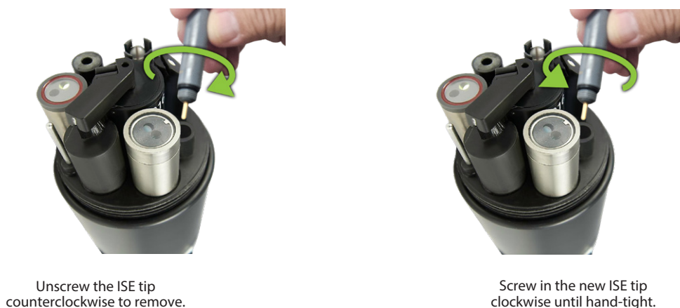
Figure 4-16 Replacing ISE Sensing Tips
