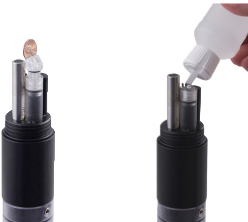
Figure 4-8 Reference Electrode Maintenance
